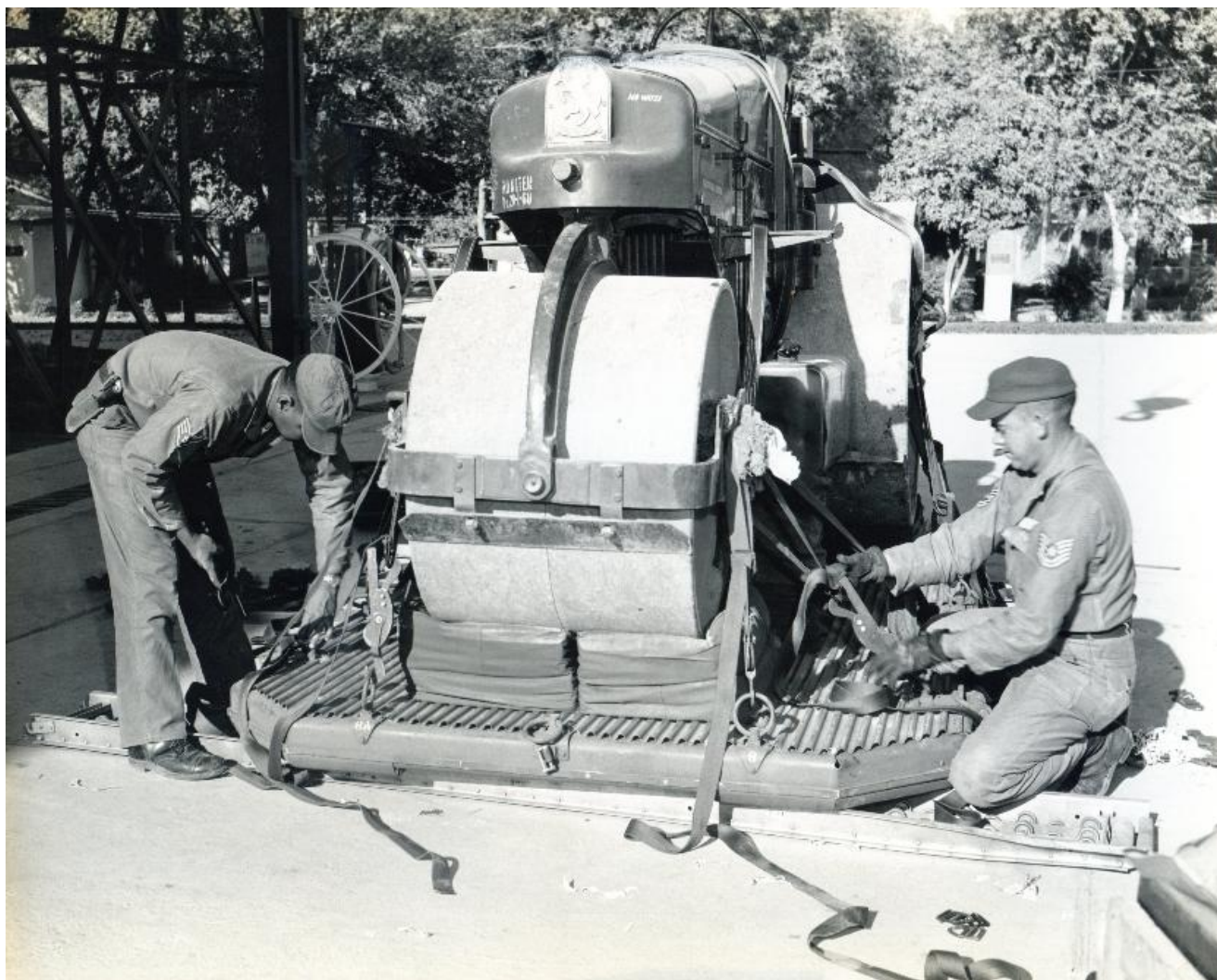
There are no photographs available of the heavy equipment drops; however this is a photo of the roller/compactor shown during pre-drop rigging at Peshawar. (U.S. Air Force Photo)
